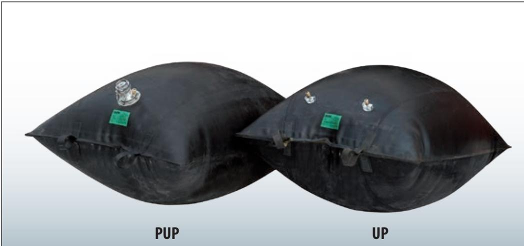
These pillow shaped pipe stoppers are mainly used in sanitary sewers and storm sewers. Their advantage is in their ability to be inserted into the pipe through standard 24" manholes. The special Kevlar reinforcement enables us to manufacture these stoppers in large diameters. The standard product line fits pipes from 40" to 88" inches in diameter.
